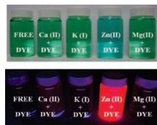
Figure 4. Digital photographs of the chemosensor solutions (5.0 \mu M) in the presence of different metal ions at 100 \mu M concentration. The upper plate is taken under ambient light, and the bottom one under UV illumination at 360 nm. Solvent: ethanol–aqueous buffer mixture (5% in ethanol, HEPES 0.1 M, pH = 7.2).
